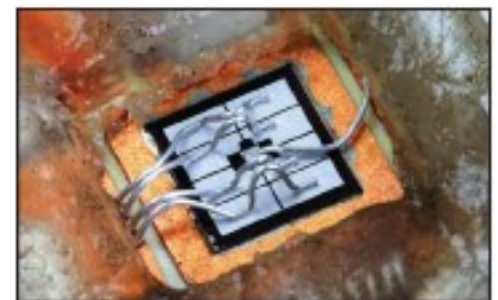
Gel Removed with FA-LIT Laser
