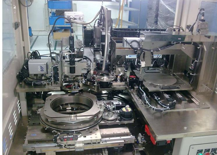
This system is designed to precisely pick and place precision lens, inspect lens' surface cosmetic defects using our in-house developed AOI, and output the good lens into wafer format tray or other types of tray for downstream process.
